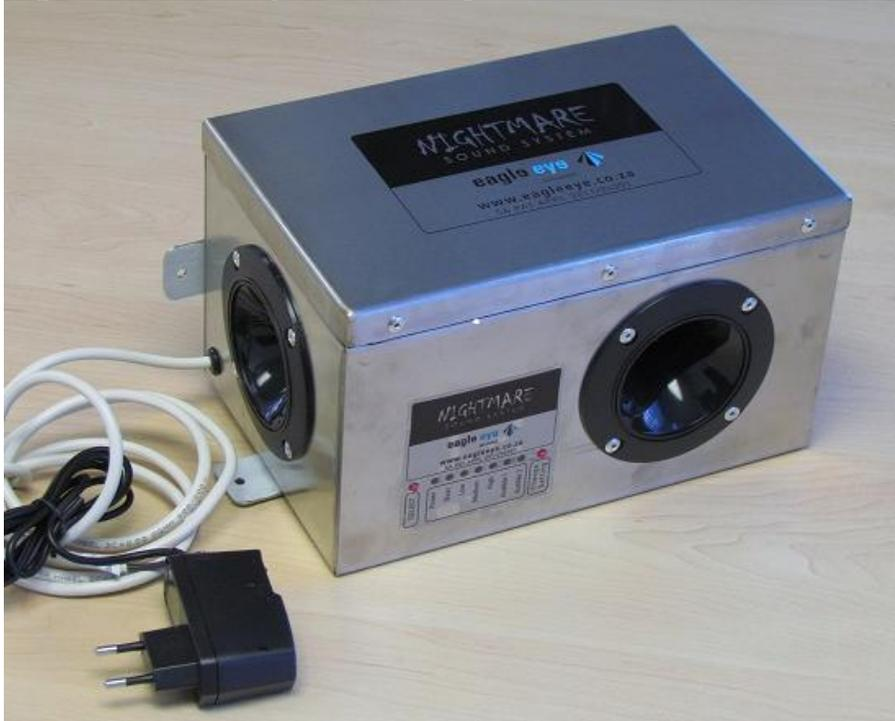
This system is ideal for open areas and warehouse applications. The sound will deter birds in a radius of 15-20 meters around the unit. (800 M<sup>2</sup> coverage in total)
